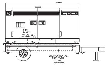
Figure 32. Internal Fuel Tank System
